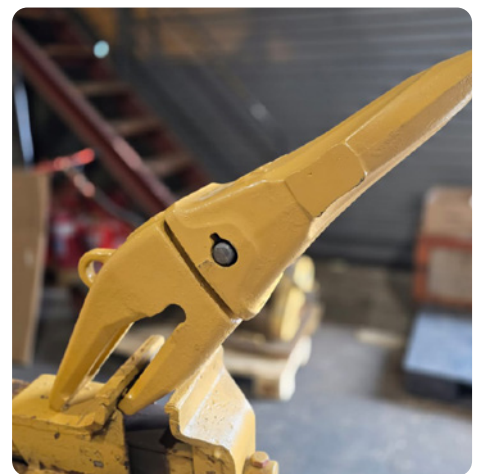
With the CapiParts Install tool , the process of tightening the pin becomes faster, safer, and controlled.
